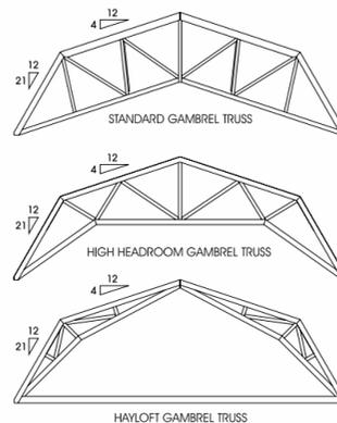
While gambrel style buildings have many practical uses, their truss design is very unique when compared to conventional buildings. The gambrel roof system is available in three types of truss designs.
